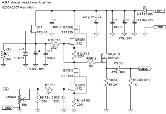
Circuit is for left channel and shared part, component numbers for Roh are in brackets.
